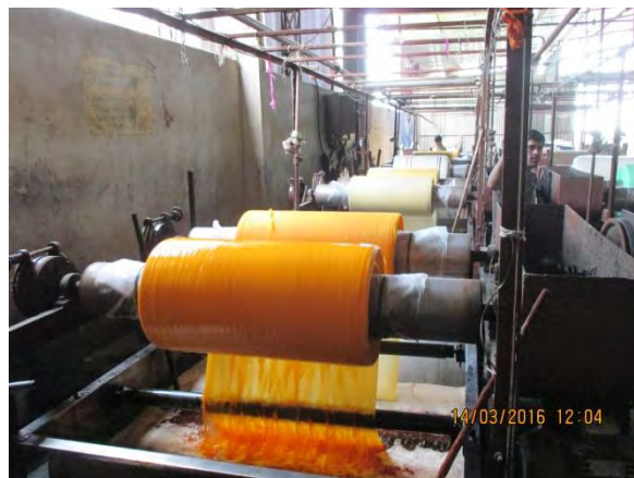
Caption: Cotton fabric dyeing using Jigger Machines
